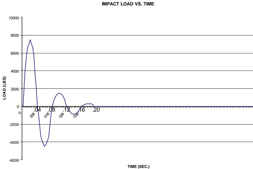
This data was obtained by attaching strain gages to the tie rod. The gage is, in effect, an electronic device which varies resistance as it is stretched or compressed. A 10 volt input is sent to the gage. The voltage output will be less than 10 V depending on how much it is stretched. The tie rod strain gage is calibrated to a load in a tensile test machine. During road load events, the voltage output is monitored and converted to loads.
