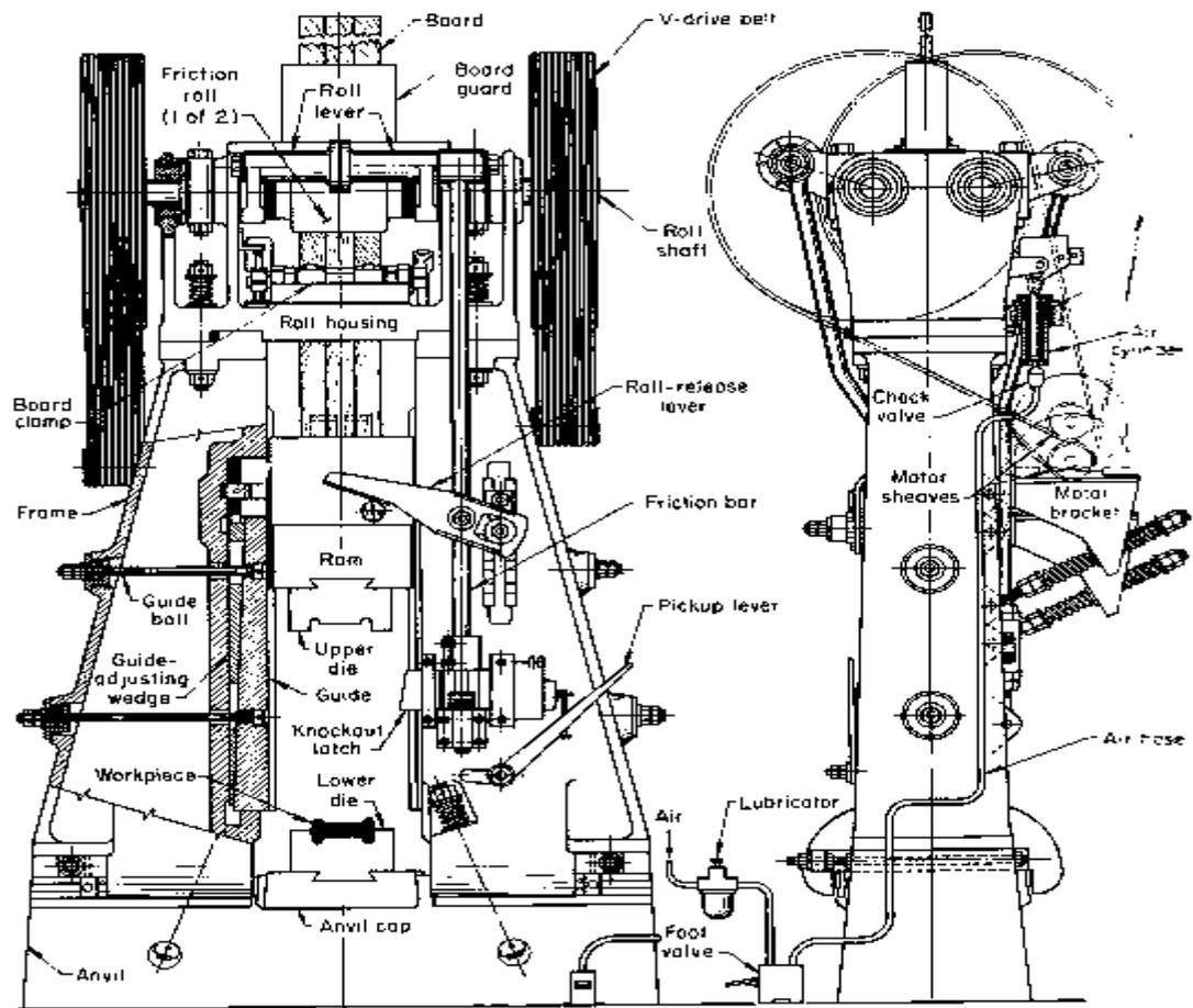
**Board Hammers** deliver their energy by gravity only. The ram is raised mechanically to a predetermined height and released. Cycle rates are high, as many as seventy per minute, and the energy imparted to the work piece is the same on each blow. Board hammers are rated by their falling weight. They range in size from 100 to 7000 pounds.
