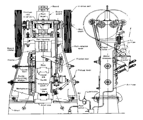
**Board Hammers** delivery their energy by gravity only. The ram is raised mechanically to a predetermined height and released. Cycle rates are high, as many as seventy per minute, and the energy imparted to the work piece is the same on each blow. Board hammers are rated by their falling weight. They range in size from 100 to 7000 pounds.
