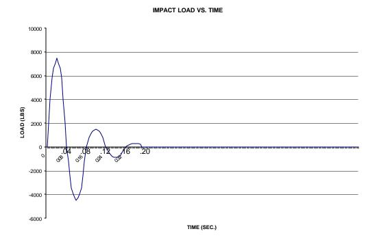
This data was obtained by attaching strain gages to the tie rod. The gage is, in effect, an electronic device which varies resistance as it is stretched or compressed. A 10 volt input is sent to the gage. The voltage output will be less than 10 V depending on how much it is stretched. The tie rod strain gage is calibrated to a load in a tensile test machine. During road load events, the voltage output is monitored and converted to loads.
