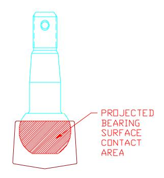
Bearing surface contact area must be sufficient to insure projected surface area does not produce stresses beyond the capabilities of the bearing material.
