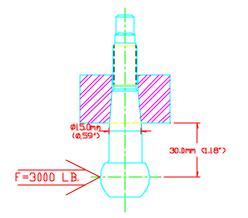
$M=3000*1.18=3540 \text{ in-lb} \\ C=0.59/2=0.295 \text{ in} \\ I=pd^4/64=.00595 \text{ in}^4 \\ R=0.59/2=0.295 \text{ in} \\ A=p*R^2=.273 \text{ in}^2$
