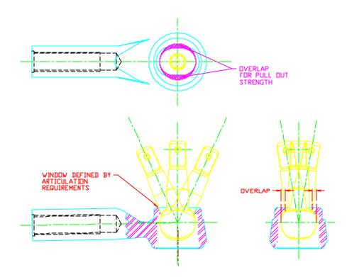
Tie Rod End Ball Sizing – Bearing Stresses
